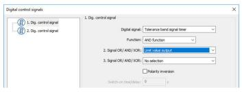
The 1st digital control signal is to be output on the PhotoMOS® relay and trigger an alarm horn once both conditions are met (timer tolerance band exceeded AND actual value over 100 °C).
