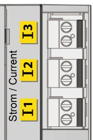
Ensure that the current transformers are assigned correctly (**I1** to **L1**, **I2** to **L2** and **I3** to **L3**) and that the energy direction is observed.
