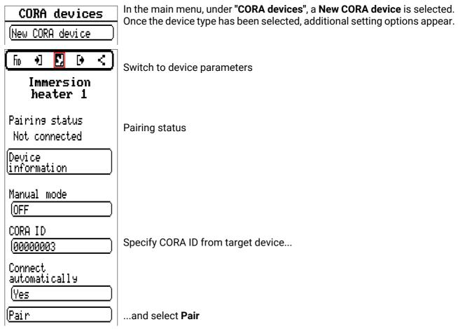
The target device must have **Allow pairing** enabled. Information about this can be found in the operating instructions for the relevant device.
