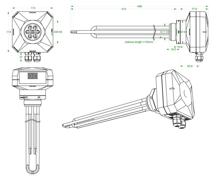
inactive length = distance from threaded head, which is not heated (120 mm)
